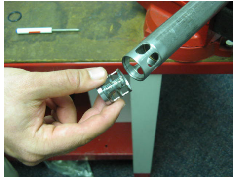
16. Remove shovel plug (Item 58) and spacer (Item 56b) from housing tube.
